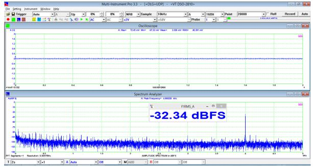
$f_s$  = 10 kHz, 44 kHz appears as 4 kHz due to aliasing, 16-Bit Mode, magnitude = -32.34 dBFS, decreased 23.24 dBFS as compared with 8-Bit Mode thanks to the adaptive anti-aliasing filter
