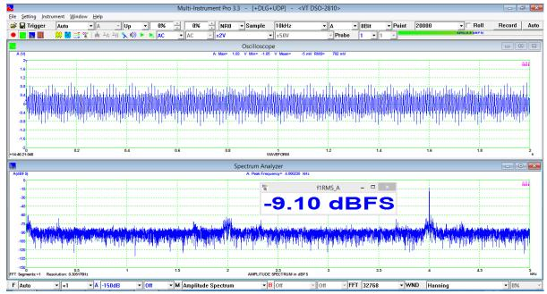
$f_s = 10$  kHz, 44 kHz appears as 4 kHz due to aliasing, 8-Bit Mode, magnitude = -9.1 dBFS
