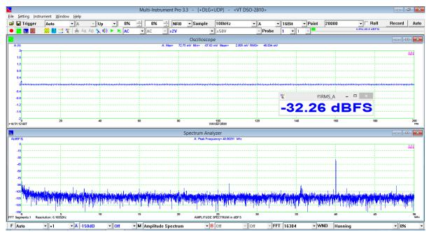
$f_s$  = 100 kHz, 440 kHz appears as 40 kHz due to aliasing, 16-Bit Mode, magnitude = -32.26 dBFS, decreased 23.24 dBFS as compared with 8-Bit Mode thanks to the adaptive anti-aliasing filter
