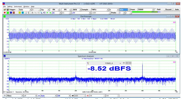
$f_s$  = 1 MHz, 4.4 MHz appears as 400 kHz due to aliasing, 8-Bit Mode, magnitude = -8.52 dBFS
