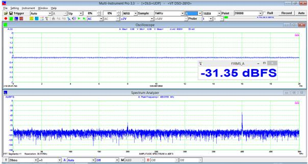
$f_s$  = 1 MHz, 4.4 MHz appears as 400 kHz due to aliasing, 16-Bit Mode, magnitude = -31.35 dBFS, decreased 22.83 dBFS as compared with that of 8-Bit Mode thanks to the adaptive antialiasing filter
